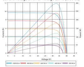
Excellent performance under weak light conditions: at an irradiation intensity of 200 W/m<sup>2</sup> (AM 1.5, 25 °C), **96.5%** efficiency (200 W/m<sup>2</sup>) is
